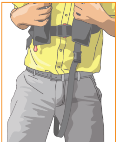
Crotch strap too loose
