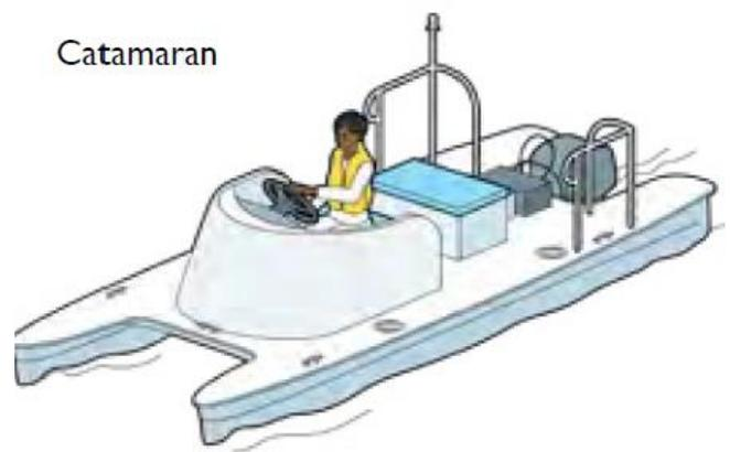
These boats are far from ideal when used as safety boats in fast flowing water because of their high centre of gravity and low lateral stability. As the boat heels then the downside sponson becomes lower in the water and the righting moment increases (as it should). However, once this sponson is immersed, then the righting moment no longer increases but decreases as the angle of heel continues to increase.
